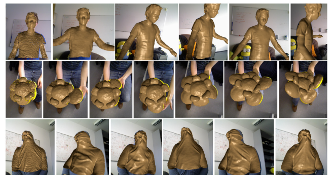
Figure 7: Similar to DynamicFusion by Newcombe et al. [NFS15], VolumeDeform by Innmann et al. [IZN*16] enables template-free non-rigid reconstruction of general dynamic scenes. The warp field is parameterized based on a fine-scale deformation lattice instead of a coarse-scale deformation graph, and sparse feature matches are integrated into the alignment objective. Image taken from [IZN*16].
