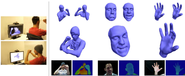
Figure 6: The first real-time template-based tracking approach that works for general objects was proposed by Zollhöfer et al. [ZNI*14]. Real-time performance is made possible by a novel hierarchical coarse-to-fine GPU optimization strategy. Image taken from [ZNI*14].
