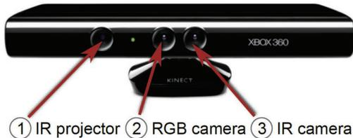
**Figure 1.1:** The Microsoft Xbox 360 Kinect: An IR projector (1) projects a unique dot pattern into the scene, which is recaptured by an IR camera (3). Depth is estimated based on the local shift between the projected and the captured pattern. The device simultaneously captures color information using an RGB camera (2).
